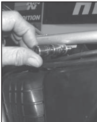
8. Remove the bolt that holds the air box to the sub-frame.
