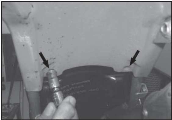
3. Remove the two lower rear fender bolts.
