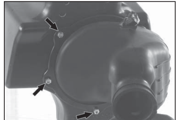
14. Remove the five hex nuts from the plate holding the intake tube.
